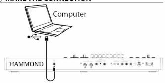
Connect the [TO HOST] port and the computer via USB "A - B" cable.
