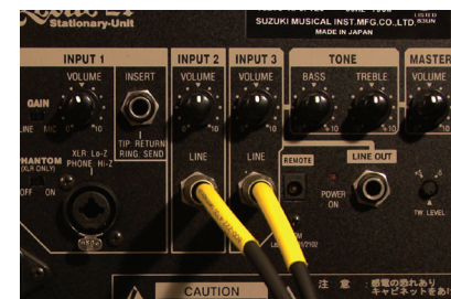
1/4 INCH CABLES PLUGGED INTO 2121 REAR
