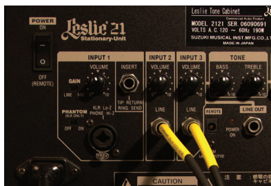
1/4" CABLES PLUGGED IN 2121 REAR
