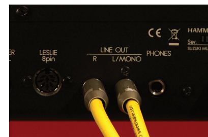
1/4 INCH CABLES IN JACKS ON BACK
