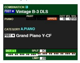
Notice the bottom line of the display now shows that the Keyboard is  $\underline{SPLIT}$ . The Keyboard is now divided into UPPER and LOWER with UPPER to the right of the Split point and LOWER to the left of the Split point. The Split point will also be shown - in this case,  $\underline{2B}$ .
