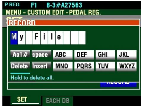
This is the screen you will use to Name your Custom Pedal Registration. You can use the FAVORITE buttons and the BANK and MANUAL buttons (the two rows of six buttons just below the Information Center Display) to select and enter characters. The data chart on the next page explains the function of each of the buttons.
