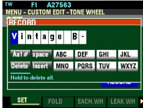
This is the screen you will use to Name your Custom Tone Wheel. You can use the FAVORITE buttons and the BANK and MANUAL buttons (the two rows of six buttons just below the Information Center Display) to select and enter characters. The data chart on the next page explains the function of each of the buttons.
