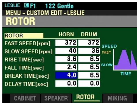
The box to the right of “BRAKE TIME” should be highlighted.
