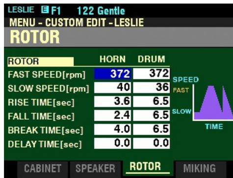
The box to the right of “FAST SPEED” should be highlighted.
