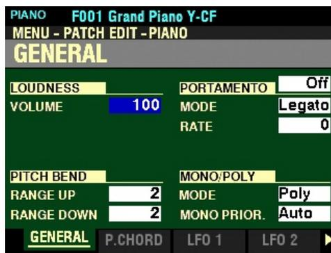
You are now in the PATCH EDIT FUNCTION Mode. You may now use the DIRECTION and PAGE buttons in conjunction with the VALUE knob to make various changes to the Patches. These changes are explained starting below.
