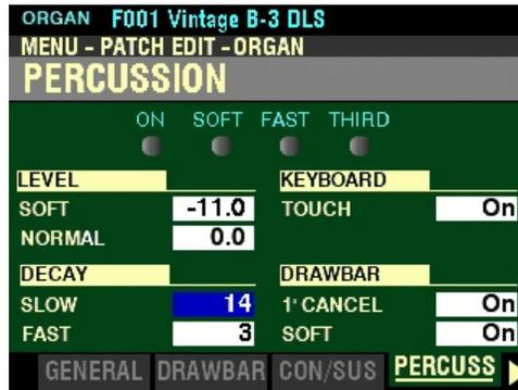
This Parameter allows you to set the overall decay (the rate at which the Percussion tone dies away while a key is held) of the Percussion tones. The SLOW Parameter sets the amount of Slow Decay (FAST button “OFF”) while the FAST Parameter sets the amount of Fast Decay (FAST button “ON”). You can set the levels separately for the SLOW and FAST Percussion Decay settings.
