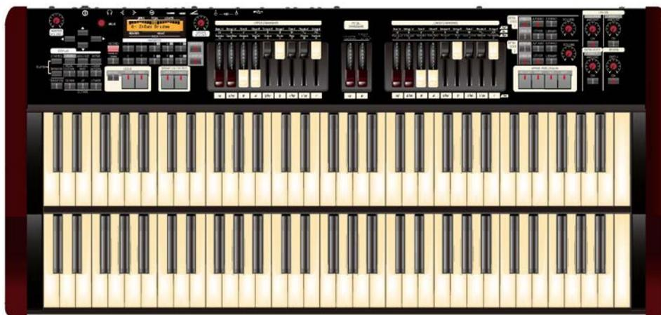
The **SKX** is a double-manual instrument which functions in a manner similar to a conventional two-keyboard organ.
