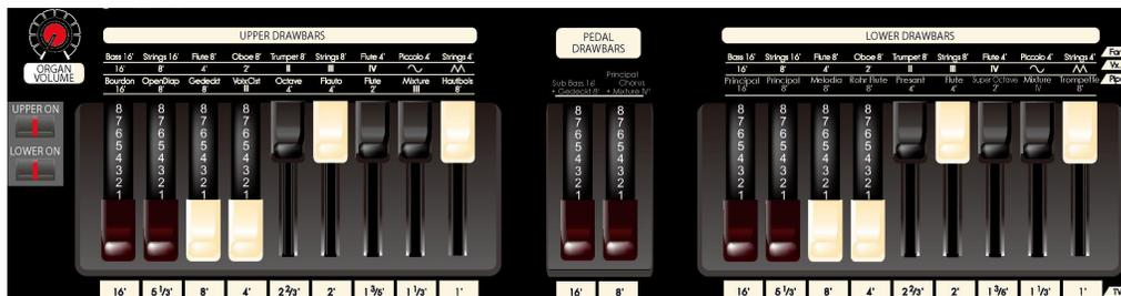
When a Patch is selected, the Drawbar settings will change internally to match the Patch. You can change the Drawbars "on the fly" for an instant edit of the Patch, but when you select the Patch again, the original Drawbar setting of the Patch will return.
