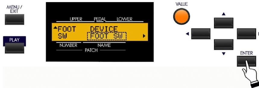
You are now in the CONTROL Edit Menu. You may now use the PAGE NAVIGATION Touch Buttons in conjunction with the VALUE Rotary Control to make changes to the characteristics of the various Controls. These changes are explained starting below.
