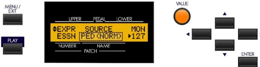
*The legend underneath the word “SOURCE” should be blinking.*
