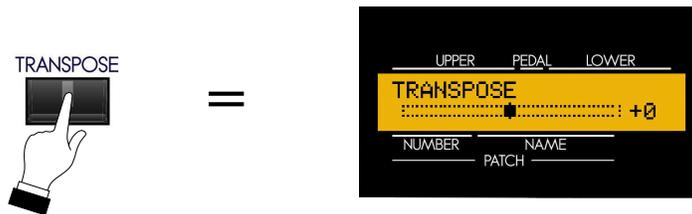
3. While continuing to hold the TRANSPOSE Touch Tab, touch the UP Touch Tab **five** times. The Information Center Display should show the following:
