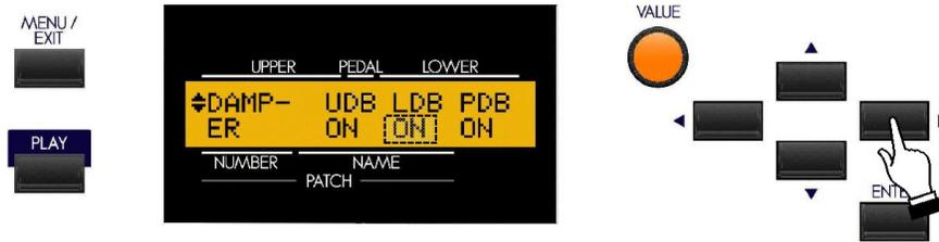
The legend underneath the word “LDB” should be blinking.
