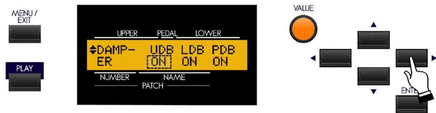
The legend underneath the word **“UDB”** should be blinking.
