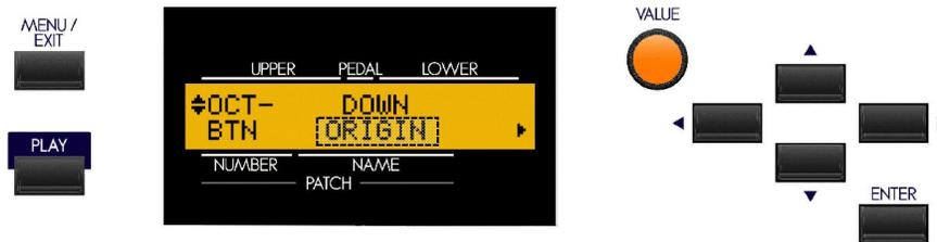
*The legend underneath the word “DOWN” should be blinking.*
